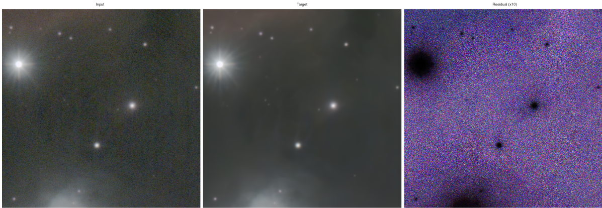
Figure 10. Residual analysis for sample frame 1 . Left: input crop. Center: target crop. Right: absolute residual (amplified 10 \times ). The residual pattern is consistent with stochastic noise removal.
