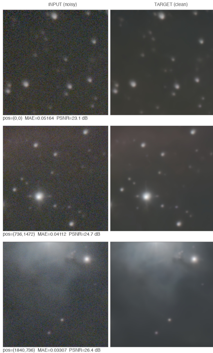
Figure 5. Input/target tile comparison for sample frame 1 . Tiles extracted at 368x368 px resolution with per-tile MAE and PSNR metrics shown.
